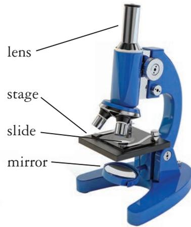
The parts of a microscope
